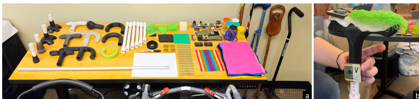
Figure 1: (a) Our co-design set-up with a modular cane, 3D printed TPU foam, laser cut decorative kerf patterns, physical interface modules, arts and crafts supplies, and an assortment of mobility aids to try. (b) A mobility aid configuration from a co-design session with an OLED display on top of the handle and a vibration motor at the base of the handle.
