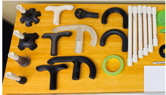
Figure 2: Parts of the modular cane, including four different types of cane tips and four handle shapes. The handles were fabricated with multiple types of materials and fabrication approaches (i.e., resin casting, thermoplastics 3D printing, and resin 3D printing)
