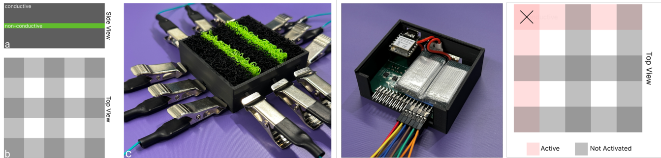
Figure 6: The design of a pressure sensor array. Two layers of conductive TPU channels are separated by non-conductive TPU.
